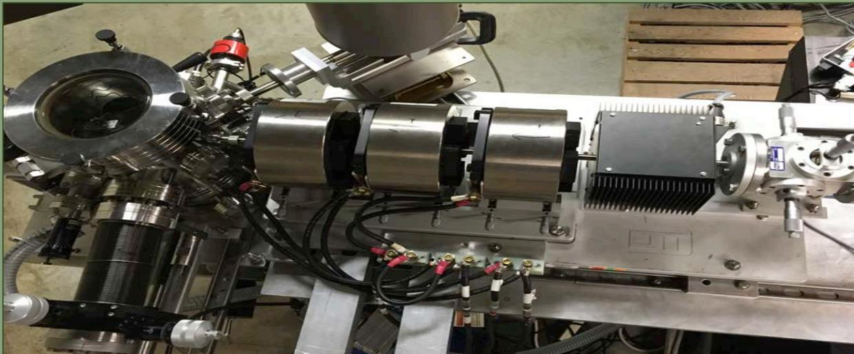
MeV ion microscope for MicroPIXE
